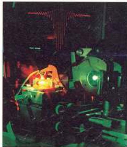
Multipass Ti:sapphire amplifier is seeded with high-quality 8-fs pulses generated by a Ti:sapphire oscillator incorporating chirped dielectric mirror for dispersion compensation.
