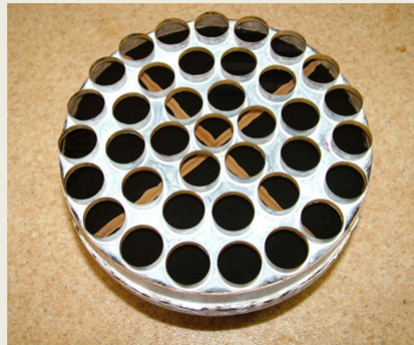
LASER MIRROR SUBSTRATES OPTICALLY CONTACTED ON GLASS TOOL ( \varnothing 30 mm, BK7)
