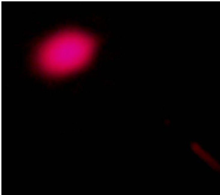
Left: Photo of a red laser beam exiting the photonic crystal fiber being connected to a 2 MHz repetition rate Yb-fiber laser with output power of 200 mW. Right: the same recorded by an IR camera
