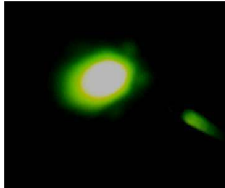
Left: Photo of a red laser beam exiting the photonic crystal fiber being connected to a 2 MHz repetition rate Yb-fiber laser with output power of 200 mW. Right: the same recorded by an IR camera
